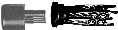
FIG. 166.—Cut-out plug used in Cook-Beach transfer system to break a false connection with a busy line.
