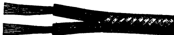
FIG. 81.—The cord of a telephone receiver. It consists of two strands of braided tinsel, insulated, and enclosed in a woven sheath. A metal pin is secured to the end of each strand, and this is inserted in the grooves of the binding-post to give electrical connection.
