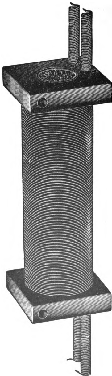
FIG. 93.—A telephone induction coil of usual size, showing the laminated core and the attachments of the primary and secondary windings.
