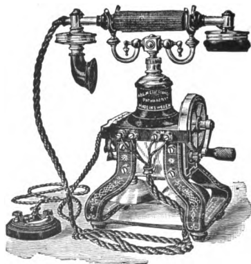
FIG. 91a.—Hand Microtelephone Desk Set, with Magneto Generator and Bell Mounted in Base.
