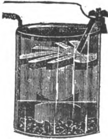
FIG. 49.—Common "crow-foot," blue-stone Daniell cell. Negative electrode, a claw-shaped piece of zinc; positive electrode copper plates, among which is disposed blue vitriol (copper sulphate).
