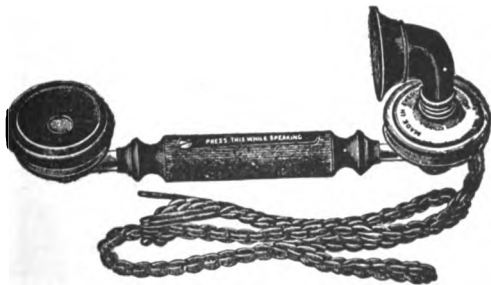
FIG. 199.—Ericsson's hand microtelephone.
