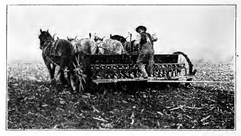
Fig. 137. A standard single-disk drill at work. This machine has 18 furrow-openers spaced 7 inches apart.
