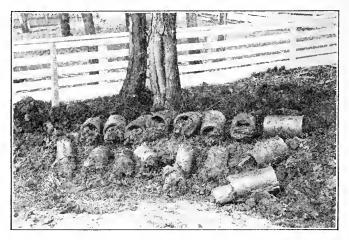
Fig. 65. A tile drain which became completely obstructed by roots from a willow tree.
