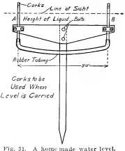
in a level line, which may be extended to a distant leveling rod by sighting over the surface of the liquid.
