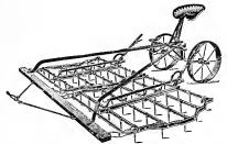
Fig. 119. A modern U-bar smoothing ard harrow of the day is harrow with protected tooth bars. A harrow cart is attached.
