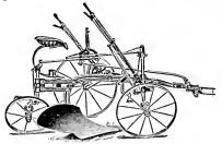
by means of bails or some similar device. This permits the plow to be lifted high out of the ground, designating it a "highlift" plow. This feature is a decided advantage for cleaning. The frameless plow has the wheels attached di-
