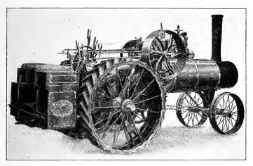
Fig. 252. A top-mounted steam tractor.
