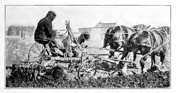
Fig. 129. A harrow attachment for a plow at work.
