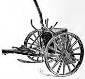
Fig. 90. Wheel scraper, dumped.
