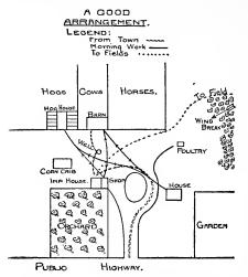
Fig. 254. A good arrangement of farm buildings. The lines of travel in doing the work of the farm are indicated.
