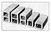
Fig. 260. Hollow clay building blocks.
