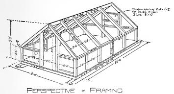
Fig. 275. The frame of the house of Figs. 271 to 274.
