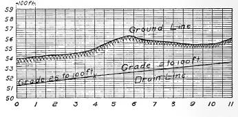
Profile of Main. Fig. 51. A profile of a tile drain.
