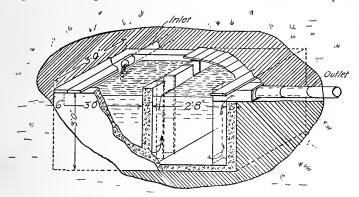
Fig. 303. A general view of a septic tank arranged to be connected with an underground irrigation or filter system without a siphon. (After Stewart.)
