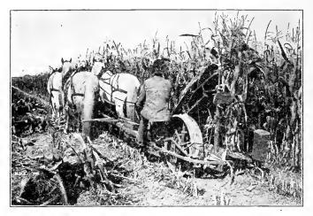
Fig. 157. A corn harvester of the vertical type at work.
