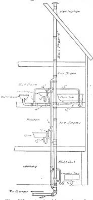
Fig. 307. A plumbing system for a two-story house. The vent plpe may be omitted with safety in country residences. (Mo. Eng. Exp. Sta. Bul.)
