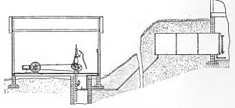
Fig. 305. An air pressure or pneumatic water supply system.
