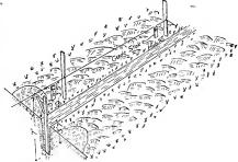
Fig. 56. The line method of grading tile ditches.
