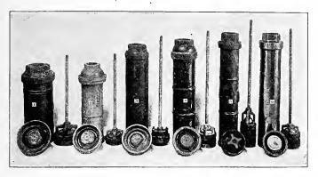
Fig. 303. Some common types of pump cylinders. 1 is of plain cast iron, 2 is galvanized. 3 is porcelain lined, 4 and 5 are brass lined, and 6 is an all-brass cylinder.
