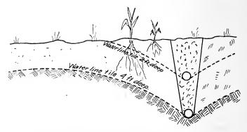
Fig. 44. Sketch showing how the ground water is lowered and the capacity of the soil as a reservoir increased by placing the tile deep.
