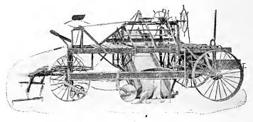
Fig. 92. An elevating grader.
