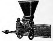
Fig. 135. An endgate seeder.
