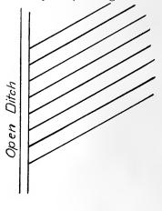
Single-Line System. 48. The single-line system of laying out tile drains.
