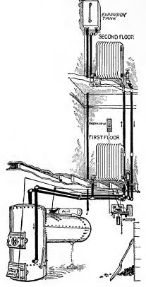
Fig. 320. A hot-water heating system. again. An expansion The locomotive type of furnace or boiler, although not in general use, is said to be quite satisfactory.
