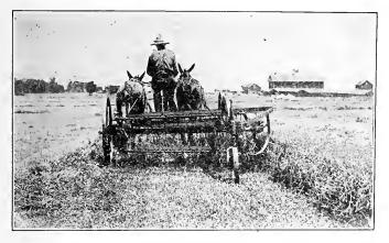
Fig. 166. A three-bar side-delivery rake at work.
