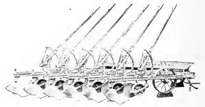
Fig. 118. An engine gang plow,
