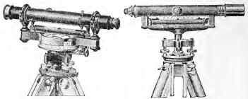
Fig. 35. A level known as a Wye level with horizontal circle and compass.
