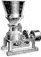
Fig. 187. A belt-driven feed mill.
