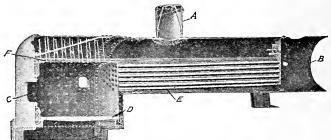
Fig. 241. A boiler of the locomotive type in section: A, steam dome; B, smoke box; C, fire box; D, grates; E, tubes; F, erown sheet.
