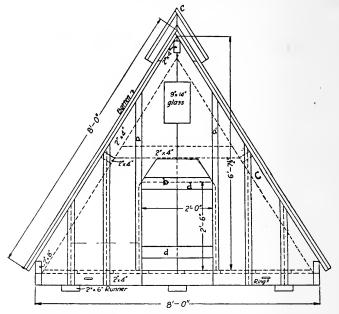
Fig. 263. Front elevation of the "A" type of colony or portable hog house. (After Wisconsin Exp. Sta.)
