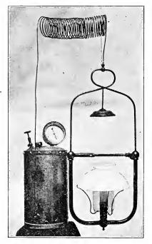
Fig. 314. A gasoline lamp. The tubing is coiled so as to appear in the picture.
