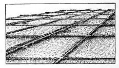
Fig. 73. Check method of irrigation. (Sep. 514, U. S. Dept. of Agr.)
