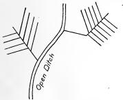
Fig. 46. The grouping system laying out tile drains.
