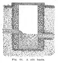
designed to provide a receptacle to catch the silt that is apt to settle at that point. They are constructed with removable covers through which the sediment may be removed from time to time. There is little doubt that these devices are very harmful in checking the flow of water in the tile, and it has been the experience of the author that these basins are never given attention when they require it.
