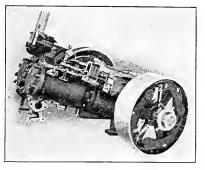
Fig. 237. The motor of an oil-burning tractor.
