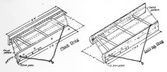
Fig. 94. Road drags made of plank and split log.
