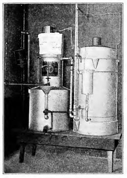
Fig. 315. A 35-light acetylene generator.
