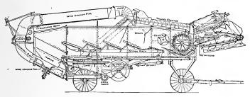
Fig. 177. A section of a modern threshing machine.
