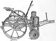
more general use than any other type. It has good penetration and is easy to guide. Where there is trash in the way, the stub runner, which hooks under the trash, should be
