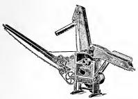
Fig. 189. two-hoe picker-A small wheel sheller equipped with self-feeder, cob carrier, and elevator.
