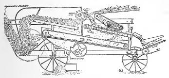
Fig. 161. A section of a corn husker and shredder.
