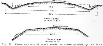
Fig. 79. Cross sections of earth roads, as recommended by the Iowa Highway Commission.
