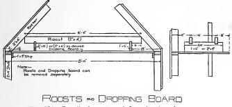
Fig. 274. Detail of roosts and dropping board.
