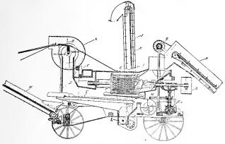
Fig. 191. A section of a cylinder sheller.
