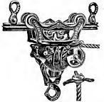
Fig. 173. A hay carrier on a steel track.
